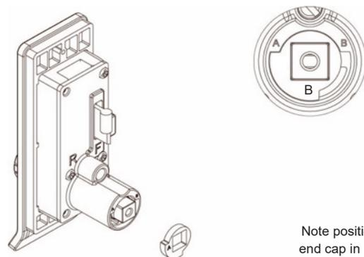
Note position of end cap in place for LH operation
